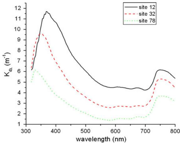
**Fig. 2** The spectral distribution of  $K_{d\lambda}$  for three sites in Lake Taihu chosen to represent average attenuation (Site 32), high attenuation (Site 12, +1 standard deviation at 500 nm) and low attenuation (Site 78, -1 standard deviation at 500 nm). Sampling site numbers correspond to those in Fig. 1
