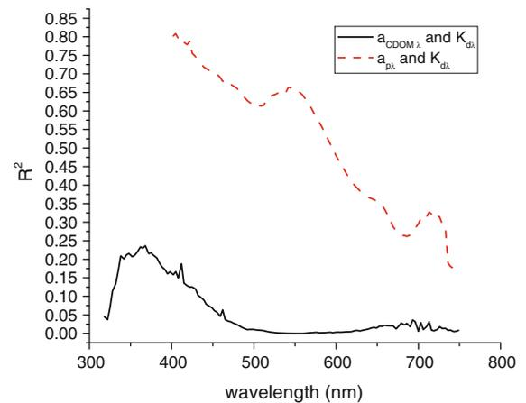
**Fig. 4** The proportion of  $K_{d\lambda}$  variance explained by CDOM and particulate matter absorption, found as the spectral variation of the determination coefficient ( $R^2$ )
