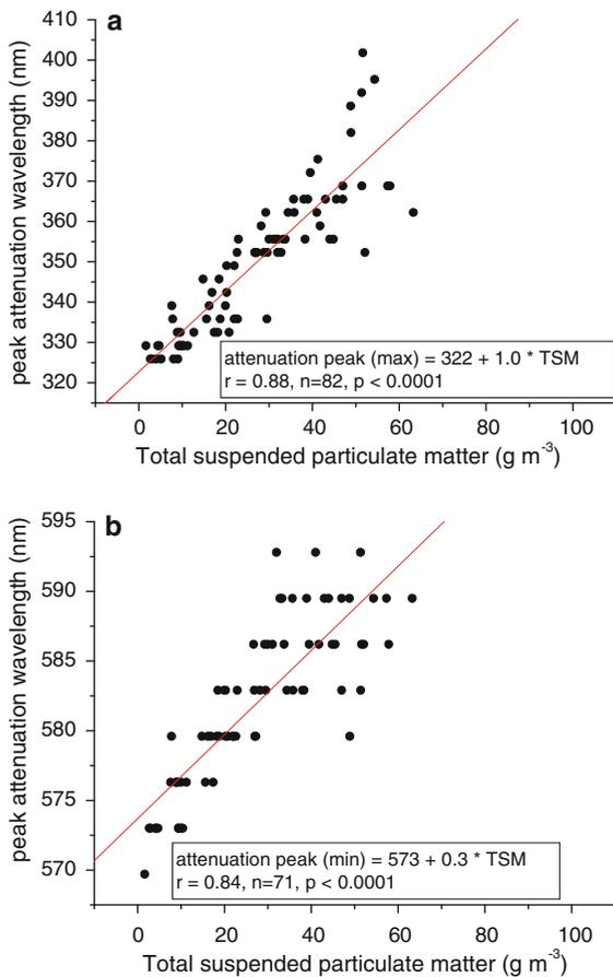
**Fig. 6** Correlations between total suspended matter (TSM) and the wavelength of maximum attenuation in the UVA wavelengths (a) and minimum attenuation in the mid-visible wavelengths (b)
