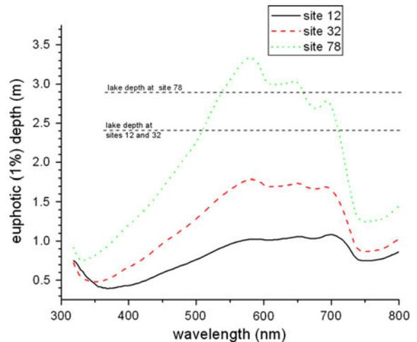
**Fig. 7** Euphotic depth (1% of downwelling solar irradiance just below the surface) and lake depth at three sites in Taihu Lake
