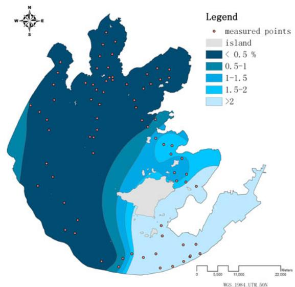
**Fig. 8** Light conditions in Taihu Lake, the percentage of subsurface downwelling diffuse solar irradiance at 676 nm reaching the lake bottom
