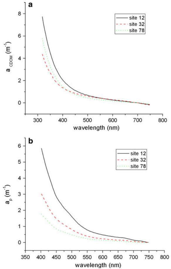
**Fig. 3** Spectral distributions of inherent optical properties at three sites of Lake Taihu in October 2008, **a** CDOM absorption (m<sup>-1</sup>) and **b** particulate absorption (m<sup>-1</sup>)
